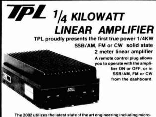
The 2002 utilizes the latest state of the art engineering including microstrip circuitry and modular construction. The three final transistors combine to produce 250W when driven by 15W or more at 13.8VDC. POWER INPUT: HARMONIC ATTENTILATION:
